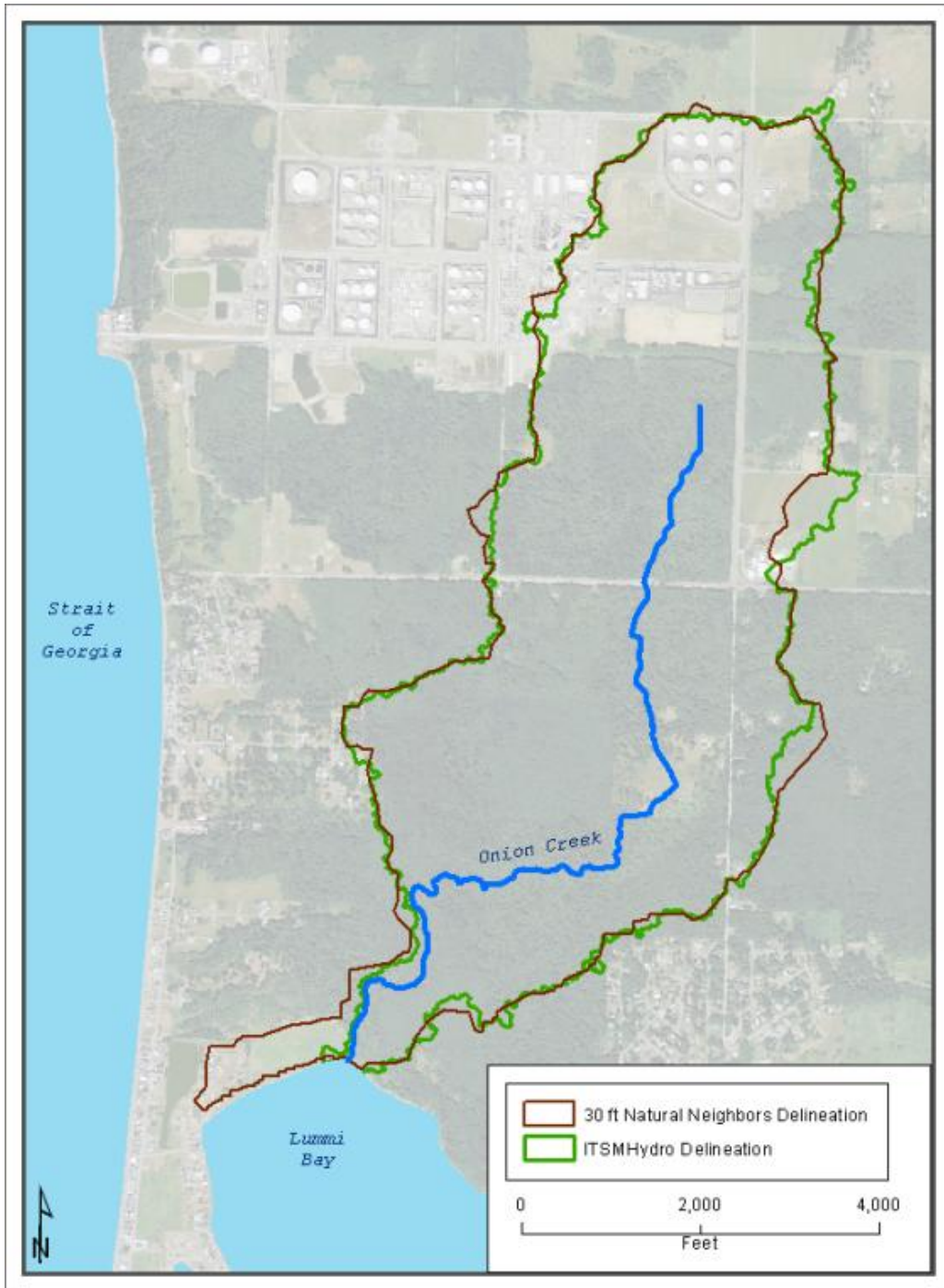
Figure 28: Test area 4 catchment comparison between the ITSMHydro delineation and a 30 ft NN raster DTM delineation using a LiDAR point appoximatly equal to the pixel density of a 30 ft pixel DTM.
