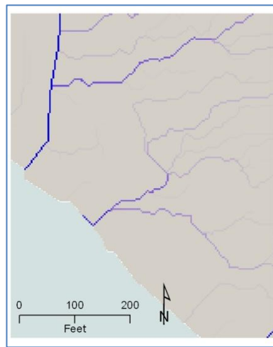
Figure 23: A typical flow accumulation surface detail; each cell stores the count of cells that pour into that cell. Higher cell counts are displayed as a darker blue.
